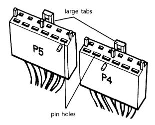
There is one 12-pin power supply socket on the right side of the main system board (toward the back) that holds both of the power supply connectors, as shown below.
